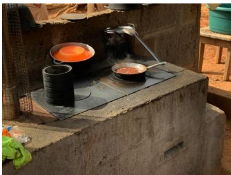
Stove installed as part of the pilot project in Nandarola
